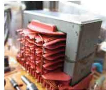
Fig. 3.4.6 Typical High Frequency Multi-Secondary Transformer
