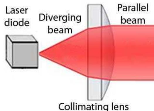
**Fig. 2.6.8 Collimating Lens**
