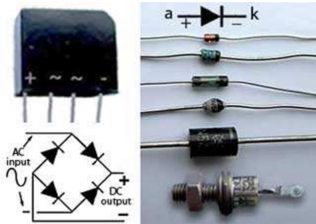
**Fig. 2.8.4 Diode Polarity Markings.**
