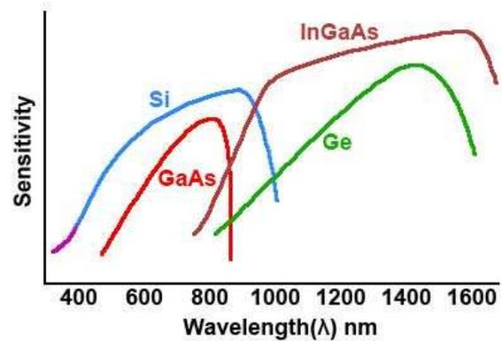
**Fig.2.7.13 Relative Sensitivity of Photodiode Semiconductors**
