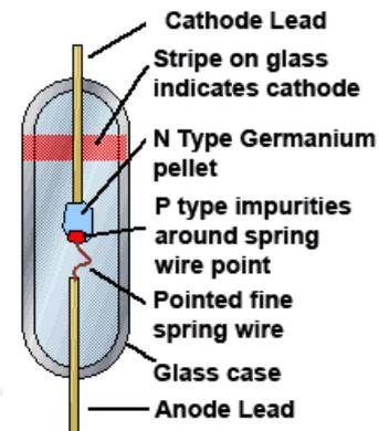
Figure 2.2.3. Germanium Point Contact Diode
