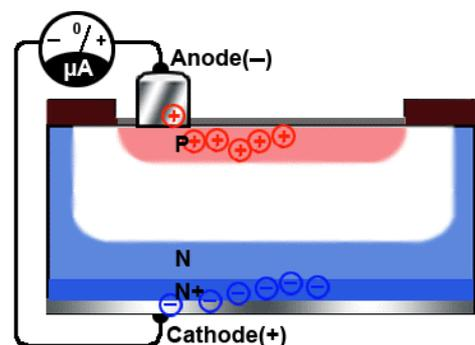
**Fig. 2.7.6 Holes and Electrons Form a Photoelectric Current**
