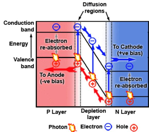
**Fig.2.7.7 Energy Band Diagram of Photodiode Action**
