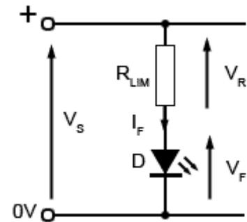
**Figure 2.5.9. LED Current Limiting Resistor**
