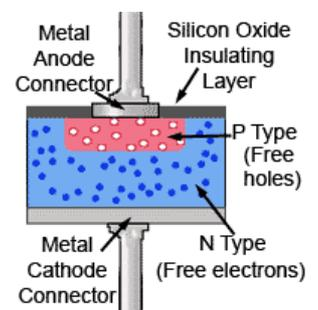
**Fig 2.0.3 Silicon Planar Diode**
