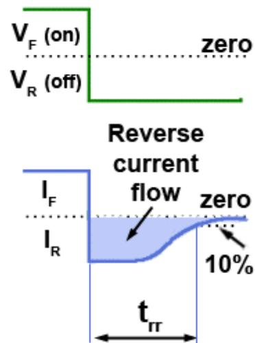
Fig 2.1.4 Reverse Recovery Time ( $t_{rr}$ )
