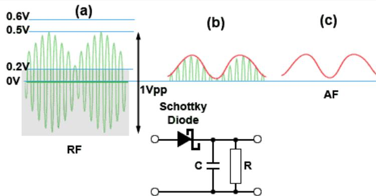
**Figure 2.2.4. AM Demodulation Using a Schottky Diode**
