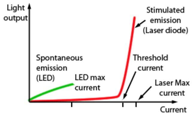
**Fig. 2.6.5. Comparison between a LED and a Laser diode**
