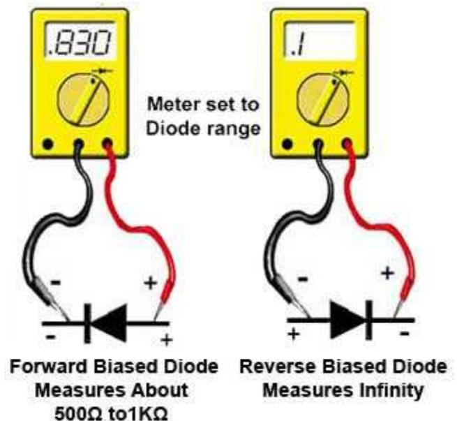
Fig. 2.8.3 Connecting a Digital Meter for Testing a Diode
