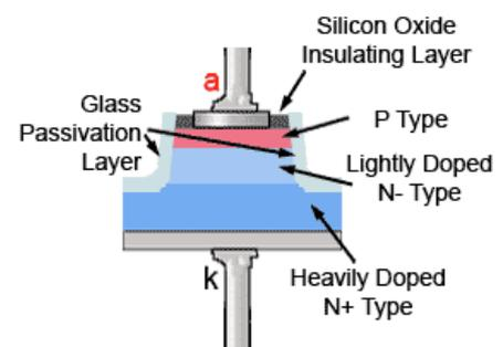
Figure 2.3.3. Simple Mesa Diode
