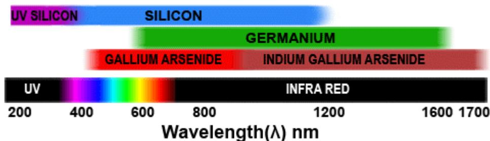
**Fig. 2.7.10 Approximate Wavelength Ranges of Common Photodiode Materials**
