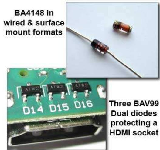
Figure 2.3.1. Small Signal Diodes
