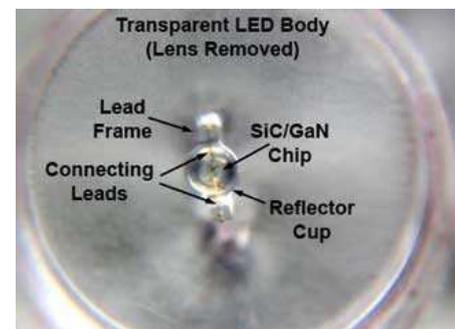
**Figure 2.5.3. LED Construction (Top View)**
