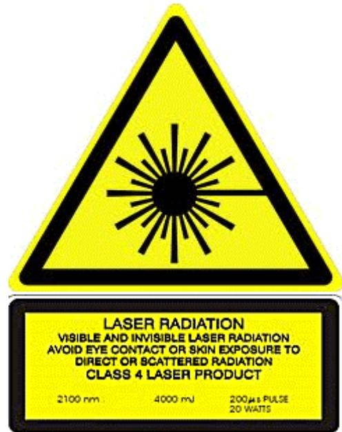
**Fig. 2.6.9 Typical Laser Warning Stickers**
