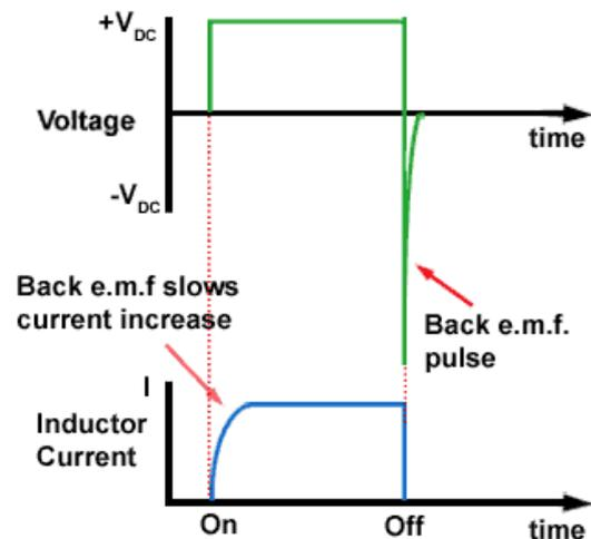
**Fig. 3.0.1 Back e.m.f. in a DC Circuit**
