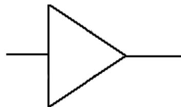
Fig 1.0.1 Amplifier general symbol, used in system diagrams
