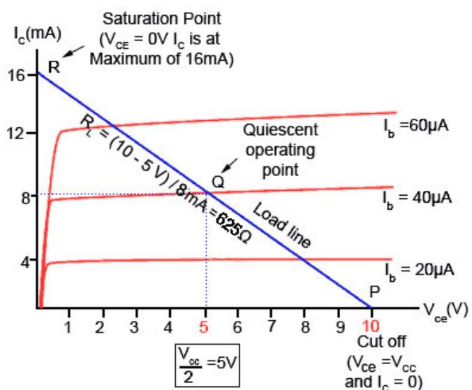
Fig. 1.2.4 Output Characteristics and Load Line
