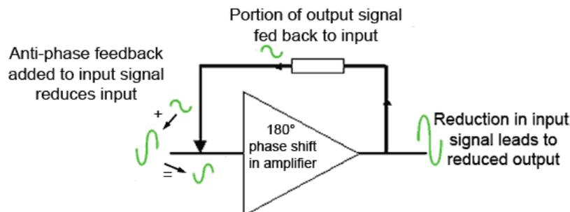
Fig. 1.1.5 Negative feedback reduces gain, distortion and noise, it also increases bandwidth.
