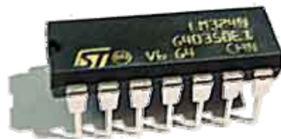
LM324N Low power Quad Operational Amplifier IC by ST Microelectronics.
