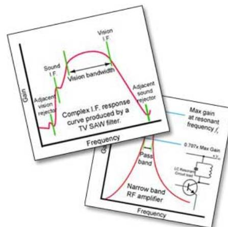
An amplifier is used to increase the amplitude of a signal waveform, without changing other parameters of the waveform such as frequency or wave shape. They are one of the most commonly used circuits in electronics and perform a variety of functions in a great many electronic systems.
