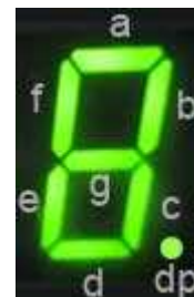
Fig. 1.6.1 Seven Segment Display
