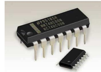
**Fig 3.2.1 Typical Logic IC Packages**
