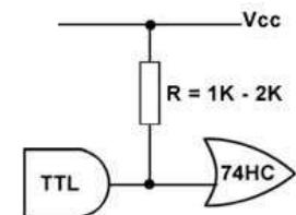
**Fig. 3.3.4 Interfacing TTL to 74HC**
