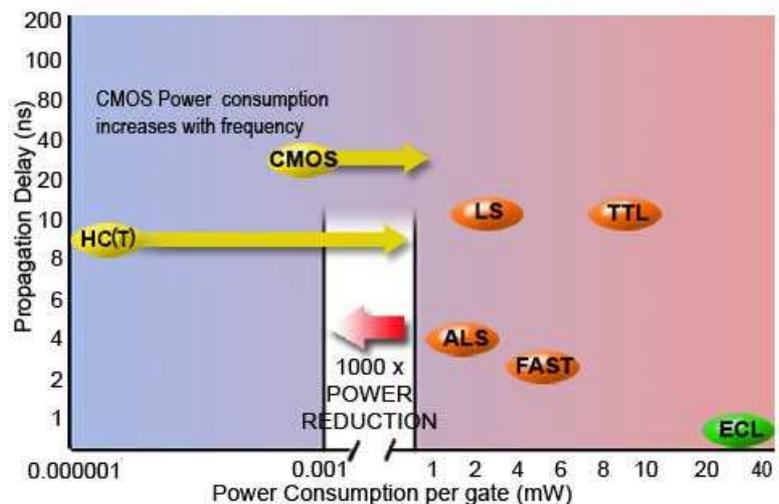
**Fig 3.1.3 Logic Families Power vs Speed**
