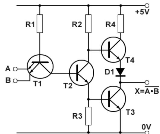
**Fig. 3.2.2 Schematic diagram of a TTL NAND Gate**
