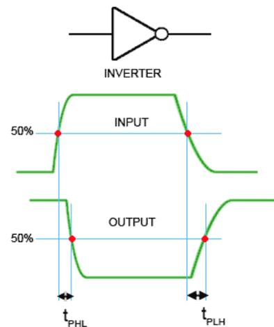
Fig. 3.2.5 Propagation Delay
