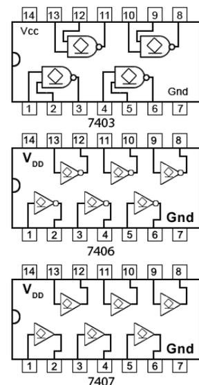
**Fig 3.4.6 Open Collector/Drain Buffer ICs**
