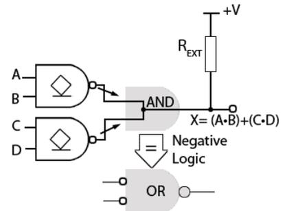
**Fig. 3.4.5 How the Wired OR Circuit Works**
