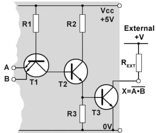
**Fig. 3.4.1 Simplified circuit of an Open Collector NAND Gate**
