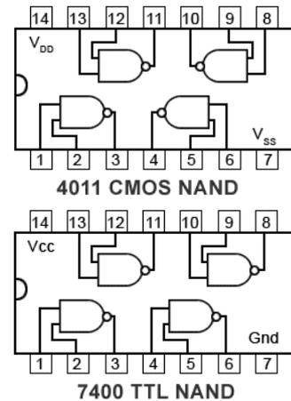
**Fig. 3.1.2 Original CMOS and TTL Pinouts for Comparable NAND gate ICs**
