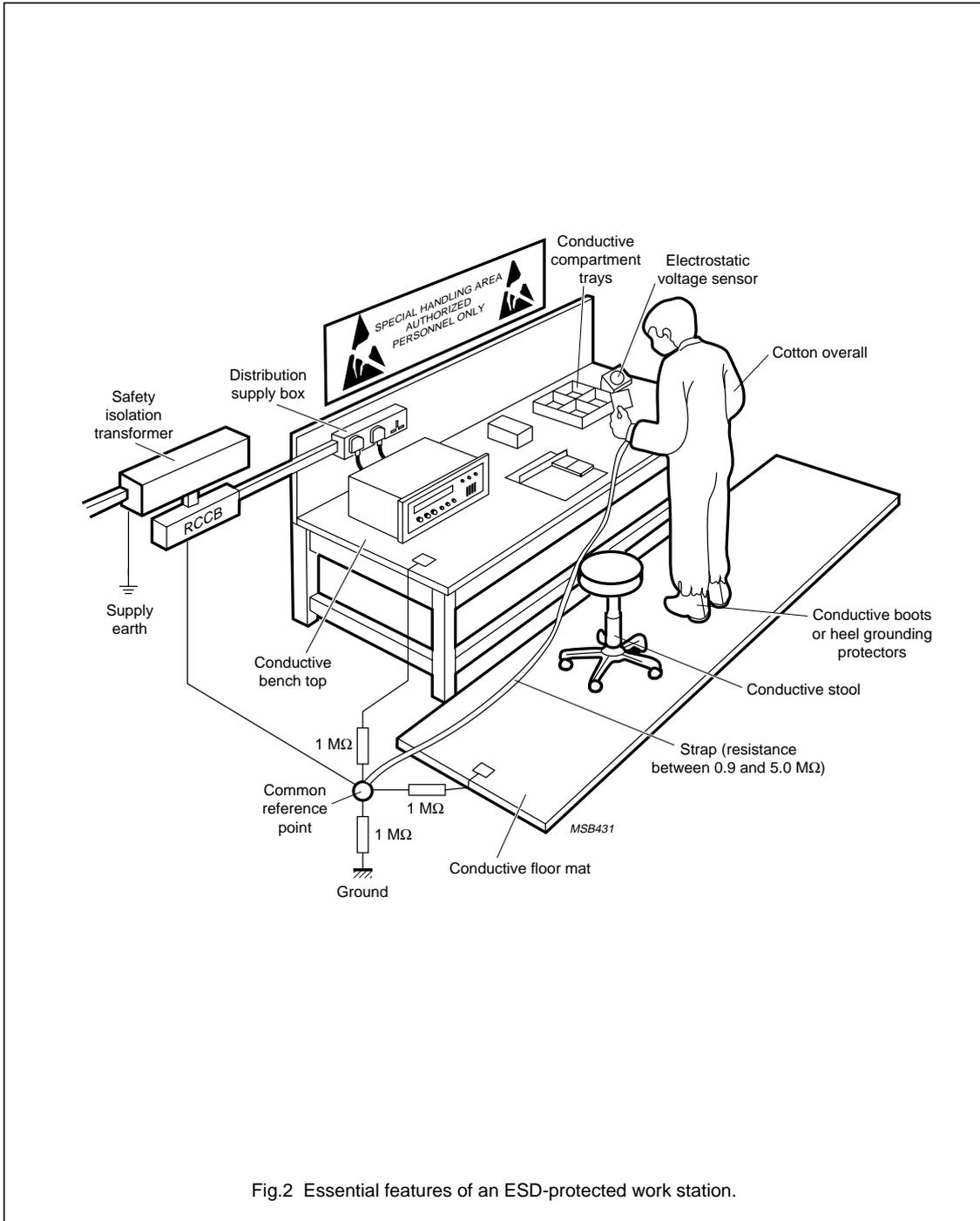
Fig.2 Essential features of an ESD-protected work station.
