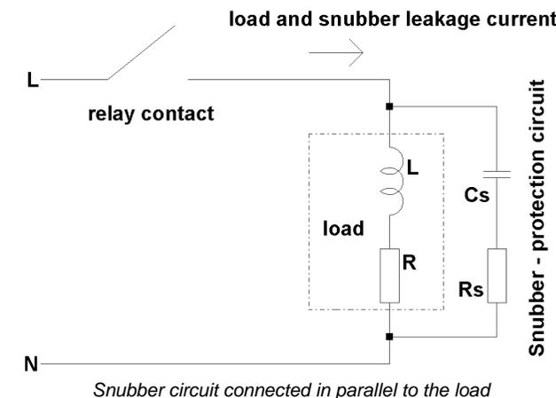
It is up to the designer to decide whether the protection circuit is connected in parallel to the switch or to the load. The sole factor to be considered in this decision is the length of time the switch is open or closed to keep the loss as low as possible. In both
