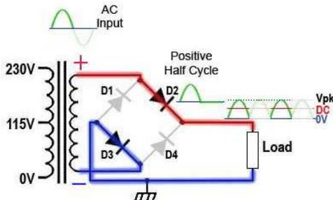
Fig. 1.1.5 Current Flow on the Positive Half Cycle
