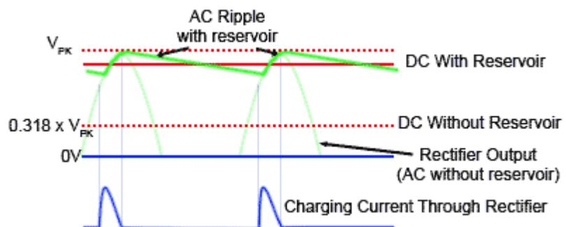
Fig. 1.2.2 Reservoir Capacitor Action
