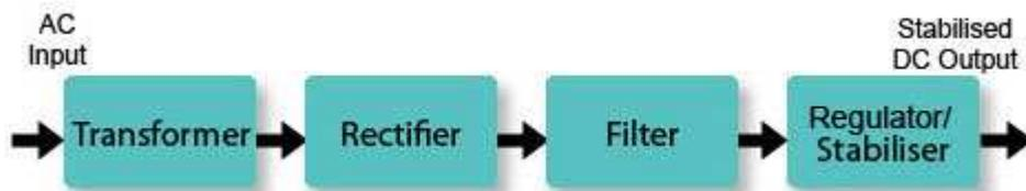
**Fig. 1.0.1 Power Supply Block Diagram**
