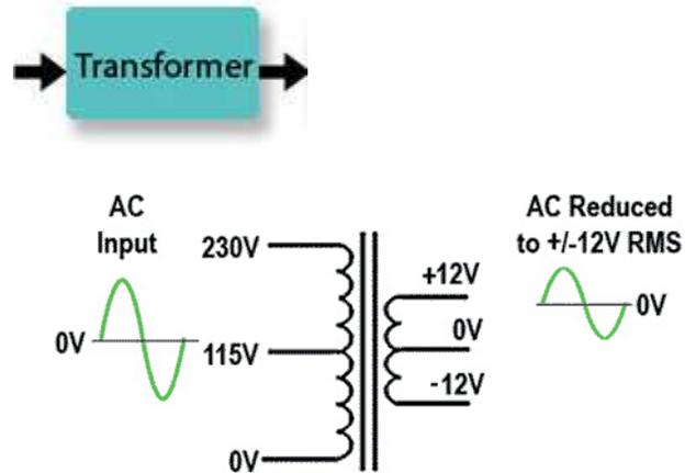
**Fig. 1.1.1 Typical Input Transformer**
