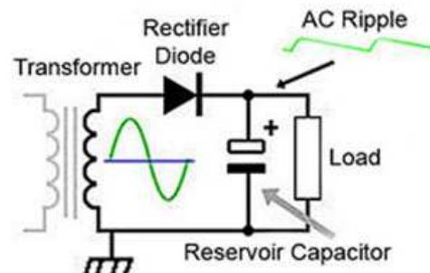
Fig. 1.2.1 The Reservoir Capacitor
