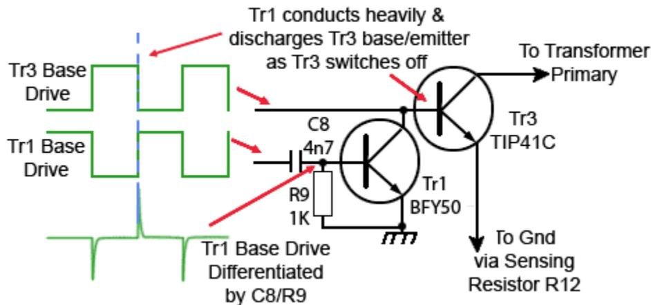
Fig. 3.4.5 Speeding up the Power Switch Turn Off
