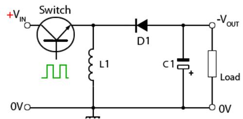
Fig. 3.1.4 Buck Converter for Negative Supplies
