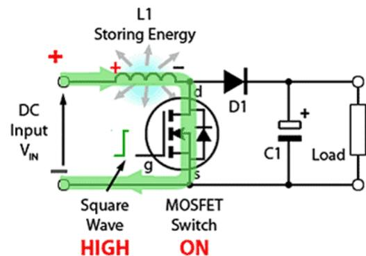
Fig. 3.2.2 Boost Converter Operation at Switch On
