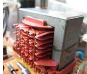
Fig. 3.4.6 Typical High Frequency Multi-Secondary Transformer
