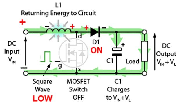
Fig. 3.2.3 Current Path with MOSFET Off
