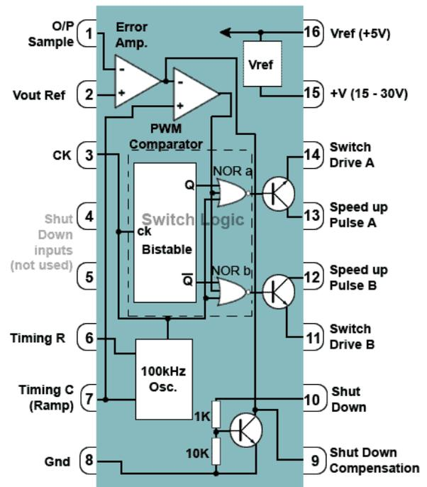
Fig. 3.4.3 The UC3524N (part detail)
