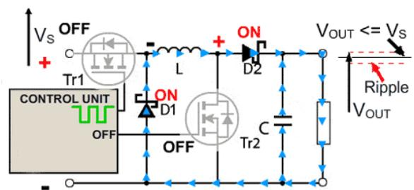
Fig. 3.3.3 Operation as a Buck Converter During Tr1 'off' Period
