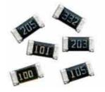
Fig. 2.3.1 SMT resistors with Three Digit Code
