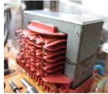
Fig. 3.4.6 Typical High Frequency Multi-Secondary Transformer
