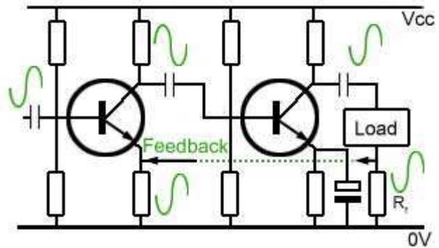
**Fig. 3.2.4 Voltage Derived, Parallel Fed NFB**
