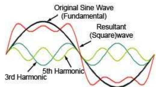
Fig. 3.4.6 The Effect of Adding In-phase Odd Harmonics
