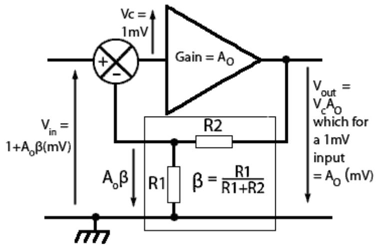
Fig. 3.1.2 Closed Loop Mode
