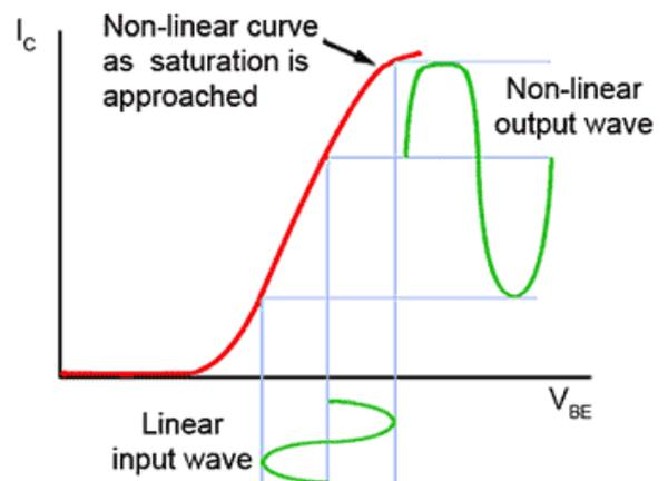
Fig. 3.4.1 Amplitude Distortion caused by poor DC biasing.
