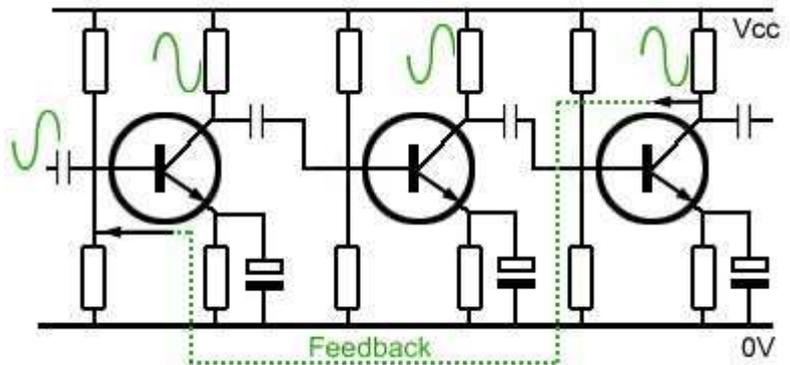
**Fig. 3.2.5 Current Derived, Parallel Fed NFB**
